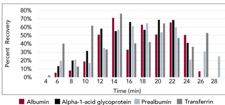
*Figure 2. Trypsin-digested protein samples were analyzed on Vanquish™ UHPLC (Thermo Scientific) over a gradient ramping from 5% to 50% solvent B (0.1% TFA in acetonitrile) over 30 minutes on a C-18 column (Acclaim 120, 5 μm, 4.6 × 100 mm). 20 μL of the sample was injected, and the flow rate was 1.2 mL/min with the column temperature held at 60°C. Percent recovery was calculated based on peak area of the extracted peptides over the non-purified peptide peak areas.*
