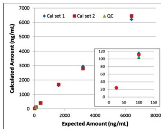
**Figure 1.** Calibration curve of THCA (25-6400 ng/mL) in negative urine using IMCSzyme<sup>™</sup>. The correction of the calculated amount with the expected amount was greater than 0.99. (Insert) The magnified region of the first two calibration points
