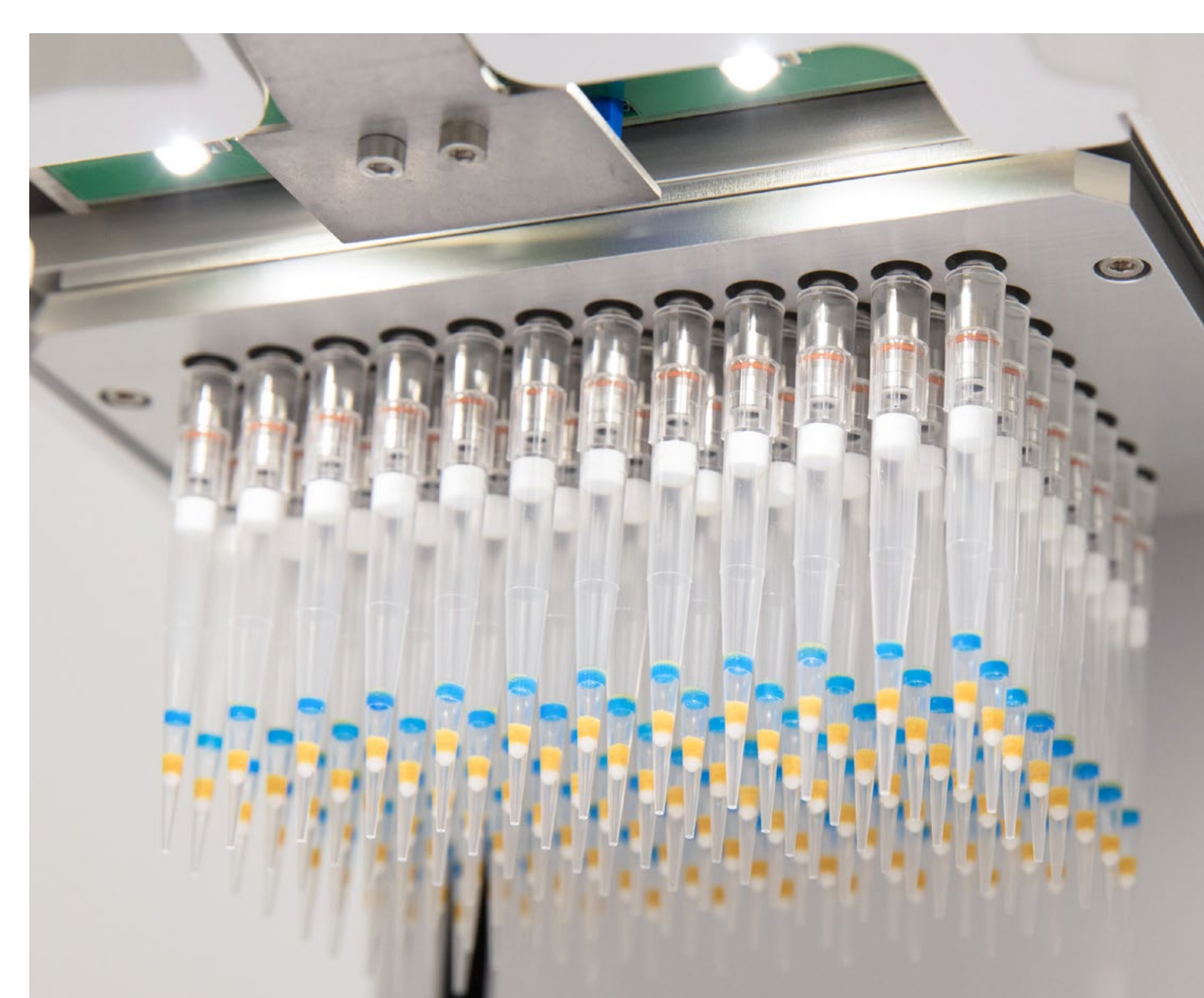
Figure 2. Desalting IMCStips with RP resin on a VIAFLO96 from Integra
