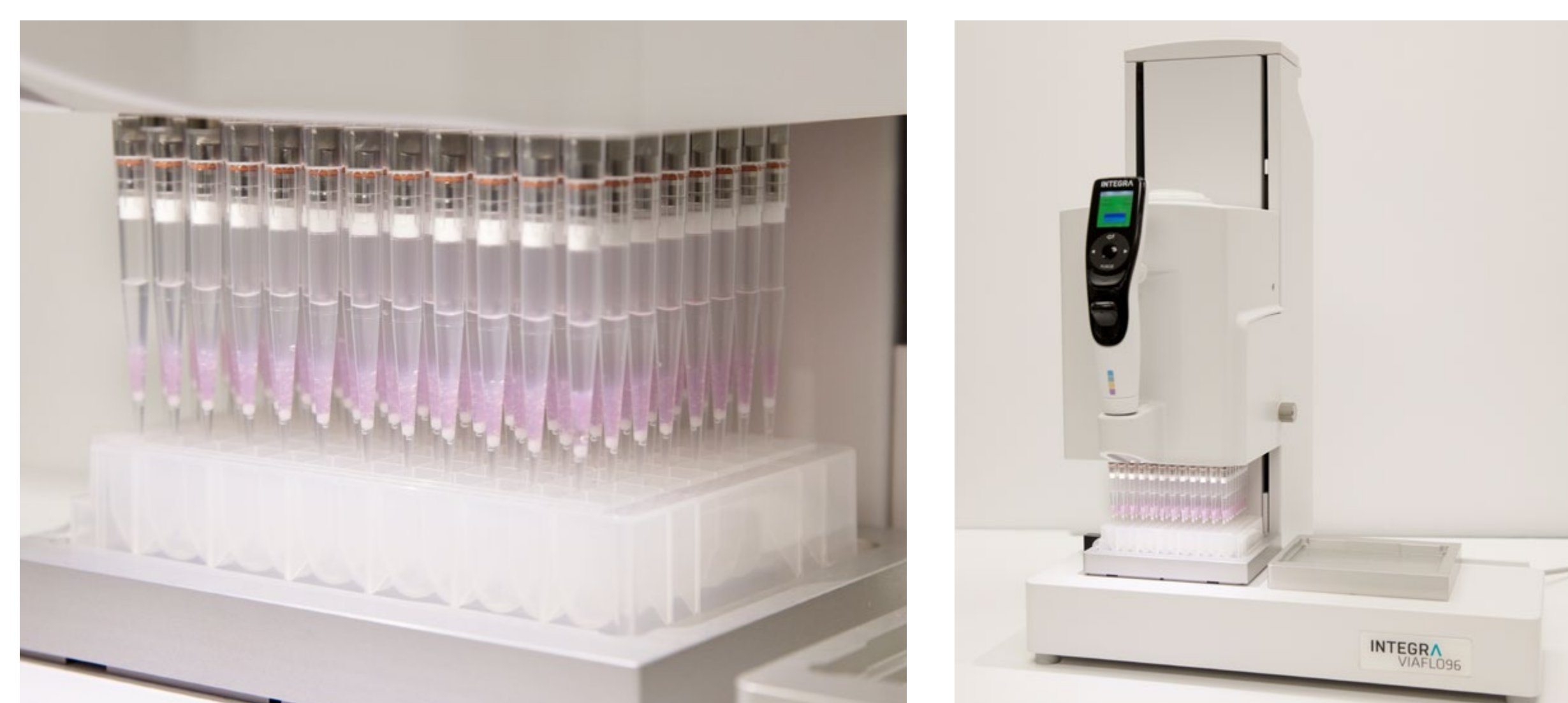
Figure 2. Affinity IMCStips with cobalt-IMAC resin on VIAFLO 96 from Integra
