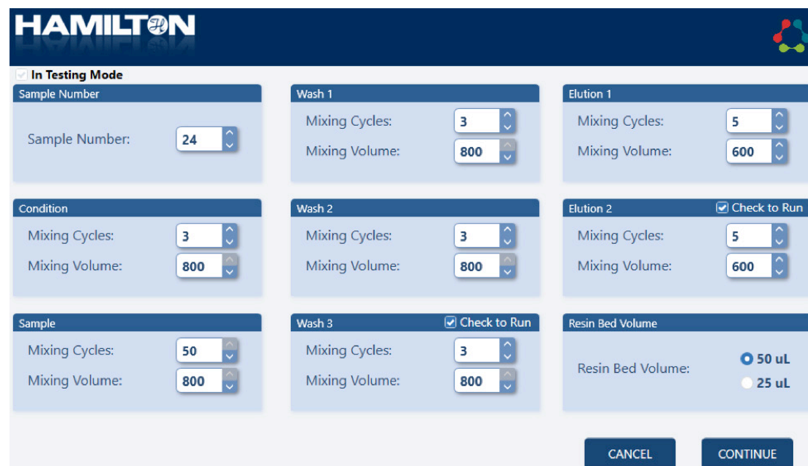
Figure 2. Graphical user interface to control aspirate and dispense cycles. Optional steps can be selected to provide easy and flexible control of the affinity purification workflow.
