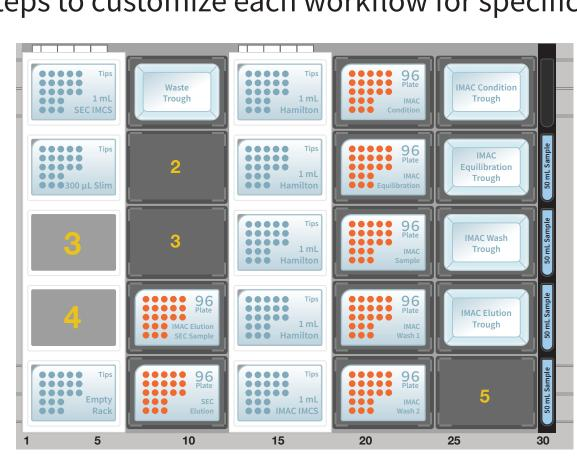
**Figure 1.** Graphical user interface to control aspirate and dispense cycles and the typical deck layout for affinity purification followed by buffer exchange.
