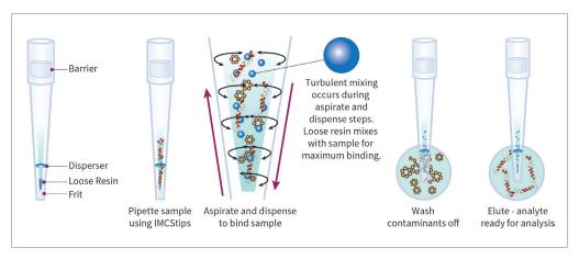
Figure 1. IMCStips use a patented dispersive solid-phase extraction (dSPE) technology. Unlike fixed-bed SPE (fbSPE) devices, IMCStips contain loosely packed resins that mix with sample solutions during aspirate and dispense cycles (mixing cycles), ensuring maximum contact between the resin and analytes of interest. Turbulent mixing within the tip is further enhanced by the addition of a patented disperser. Purification follows a typical bind, wash, elute workflow.
